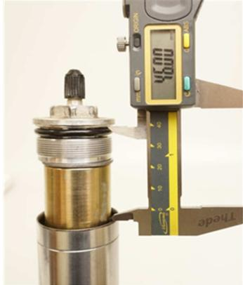
2B. If you have a cartridge fork with an external top-out spring the cartridge rod does not need to be attached to the cap for this process.
